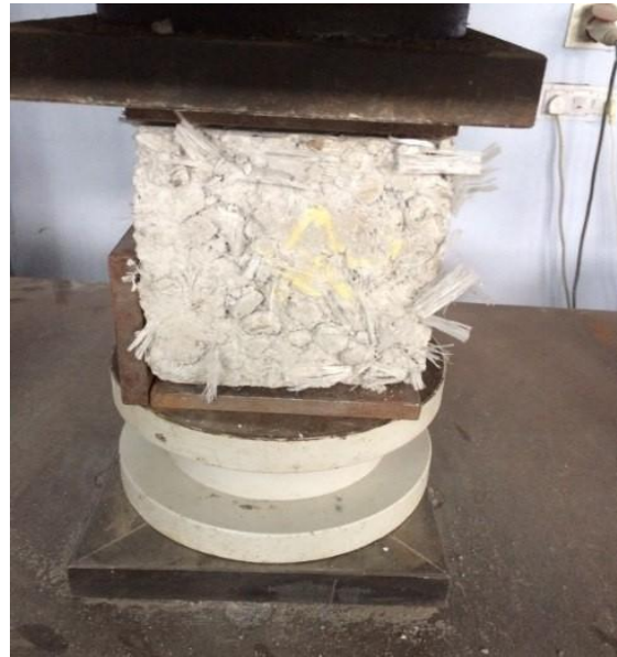
Figure 3: Splitting tensile strength testing using UTM
